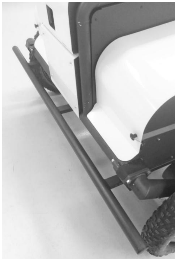
Figure 4 – Shock Absorber/Emergency Stop
