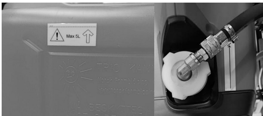
Figure 20 – Warning Labels for the External Fuel Tank
