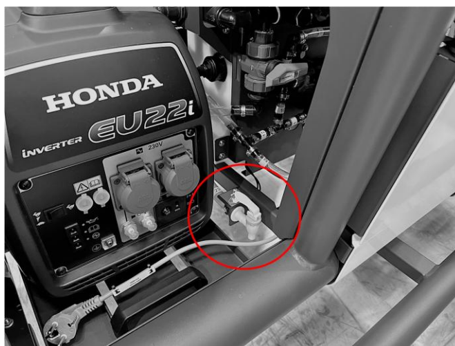
Figure 6 – The Water Tap is Located Between the Generator and the Tank
